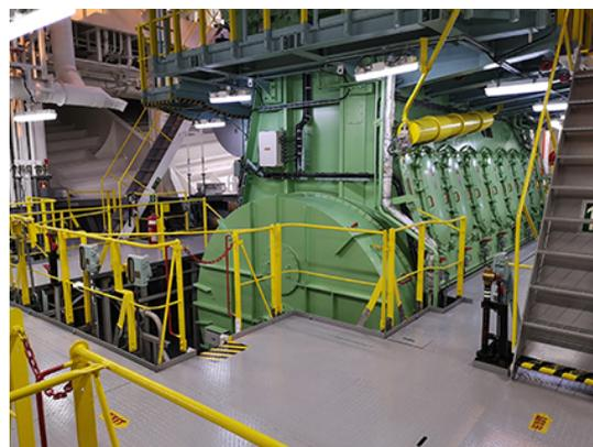
*View of the first-generation MAN B&W ME-LGIM engine aboard the 'Mari Jone', the dual-fuel, methanol-powered tanker that Waterfront Shipping took delivery of in 2016. As can be seen, the engine room is noticeably spotless (picture courtesy Marininvest)*
